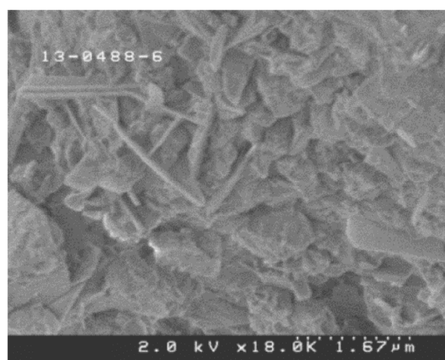
Figure 1. Scanning electron microscopy (SEM) images of two cement particles. Left: cement with minor prehydration – the cement surface is mostly smooth and free of hydration products. Right: cement with severe prehydration – the surface is completely covered with a dense layer of hydration products that will act as a barrier, reducing the reactivity of the cement when mixed with water.
