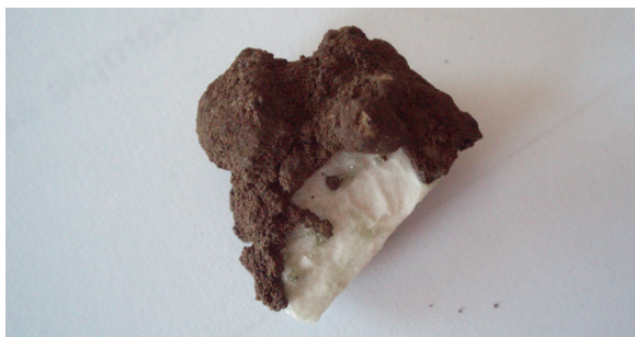
Figure 1. When things go seriously wrong: a lump of clinker with a piece of RDF embedded.
